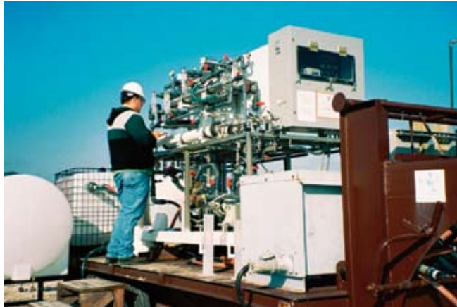
Figure 1. Portable Desalination Unit for On-Site Testing
