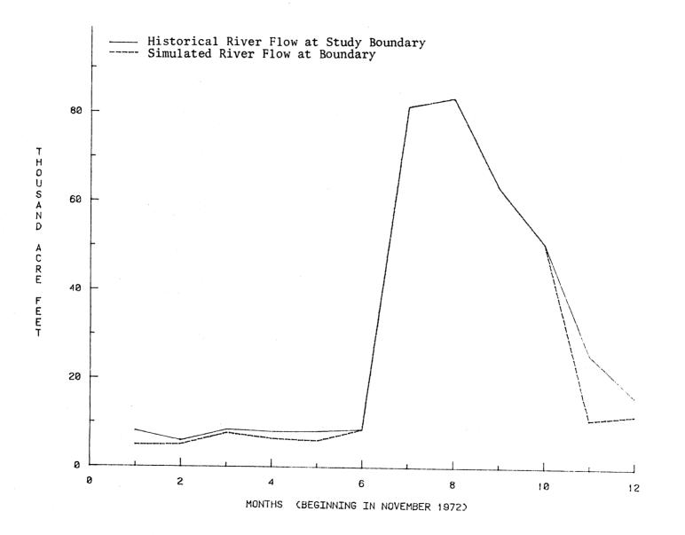
Figure S-4. Computer Simulation Flows vs. Historical Flows after Model Calibration
