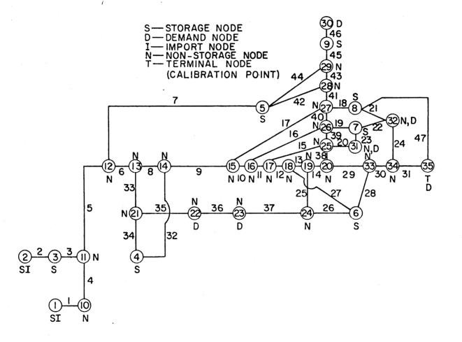
Figure 11. Link-Node Configuration for the Rawhide Case Study
