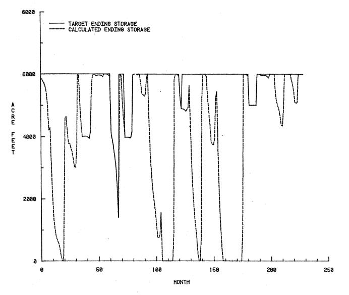
Figure 30. Target vs. Calculated Storage Levels for Long Draw Reservoir
