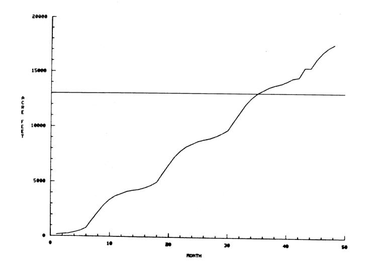
Figure S-5. Accumulated Reusable Effluent Deliverable to Rawhide Cooling Pond
