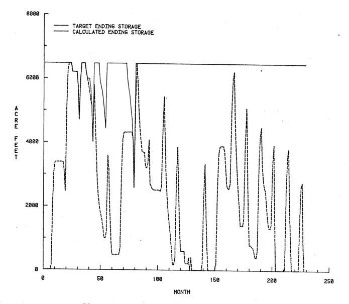
Figure 29. Target vs. Calculated Storage Levels for Joe Wright Reservoir
