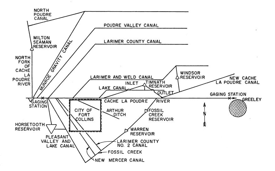
Figure 6. Detailed Schematic of Diversion Canals in the Upper Basin
