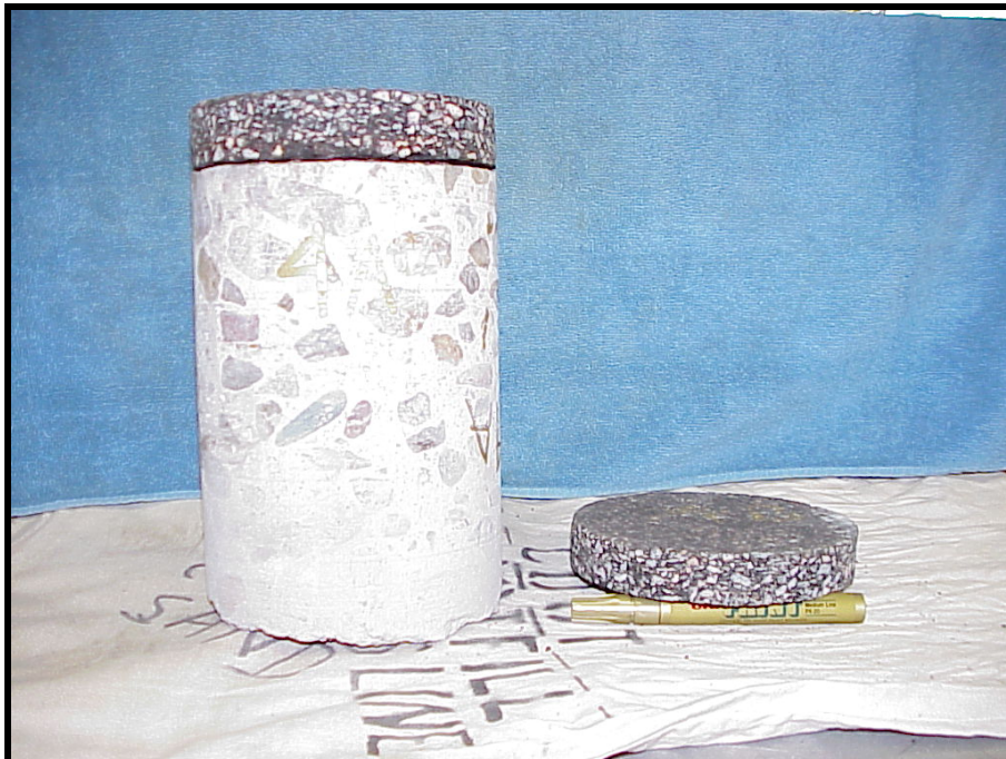
Figure 19: Core sample 4A from coring site 4
