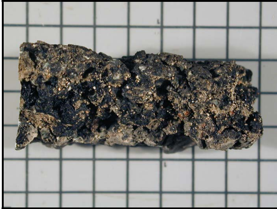
Figure 39: Core sample with evident striping and moisture damage
