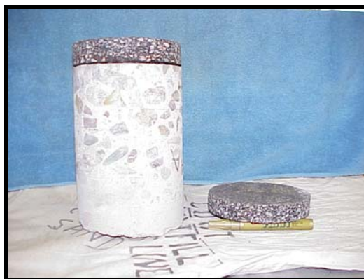
Figure 2: Core sample 4A SMA over PCCP
