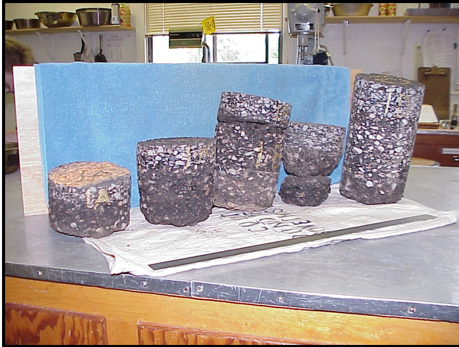
Figure 15: Core samples 2A,2AB,2B,2C,2CC from coring site 2
