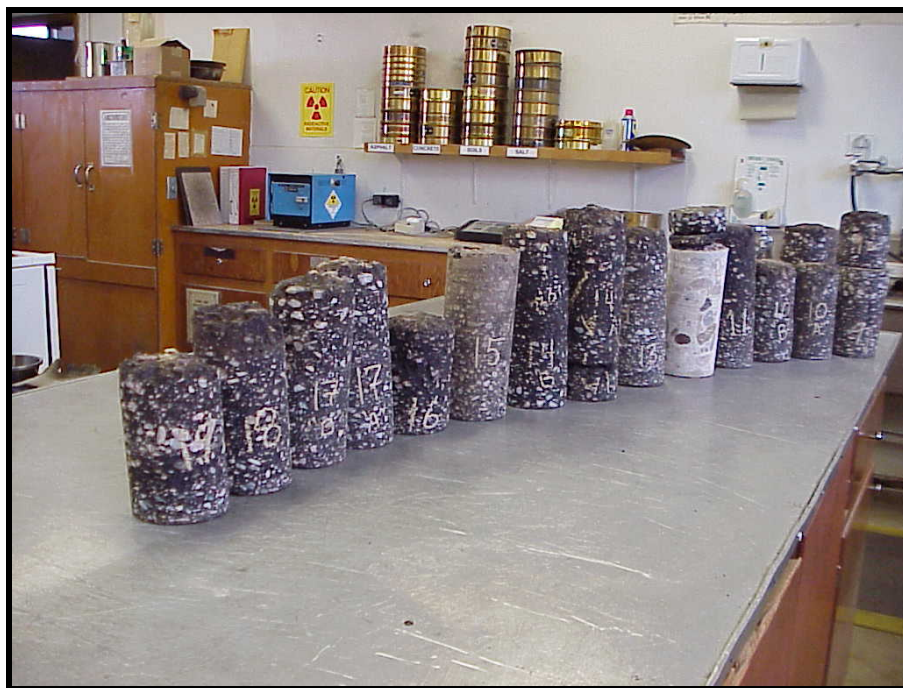
Figure 13: Coring samples 9 through 19 taken for 2001 rehabilitation
