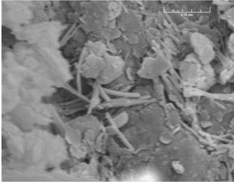
Figure 8-C. Scanning electron microscope image of ettringite distribution in soil C2 with 0.8 percent sulfates and after 28 days cure.
