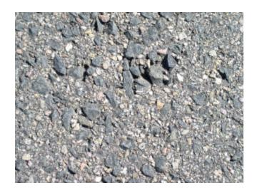
Figure 13. Photograph of core taken over a top-down crack. This crack was only found in the top mat; it was not apparent in the lower mat. Although it is not well defined it does appear that the material around the crack is coarser than the material on either side of the crack.
