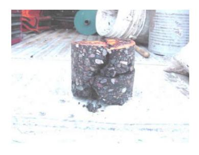
Figure 6. This crack is reflective, as it goes through the entire thickness of the pavement
