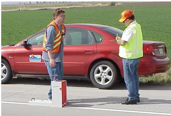
Figure 5. The Delta LTL2000 measures retroreflectance in any light condition.
