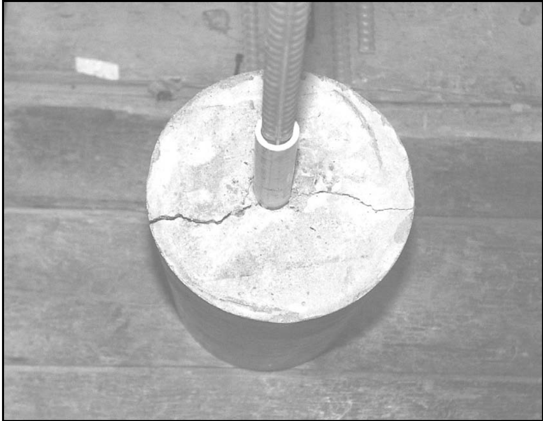
Figure 2.9 Concrete splitting during pullout
