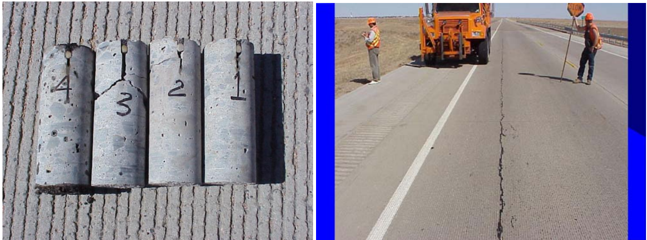
Figure 24: Cores Showing Non-Working Joints
