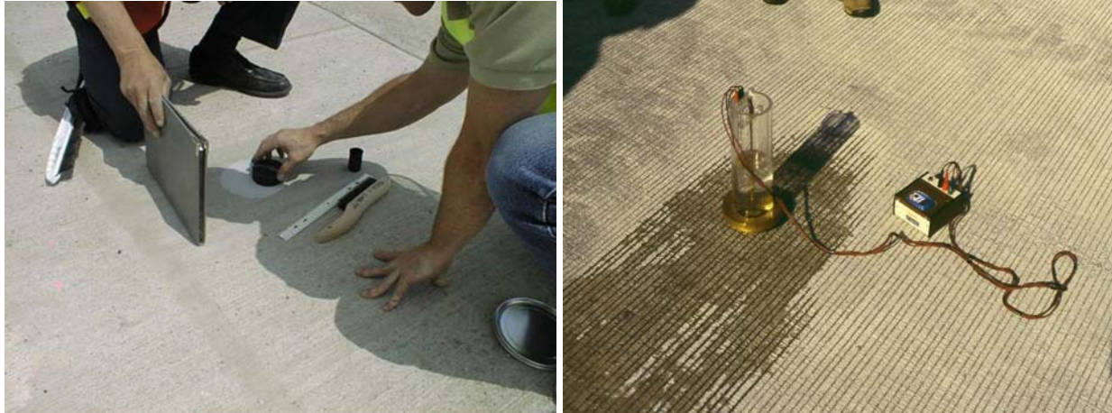
Figures 5 and 6: Sand Patch and Outflow Meter Testing
