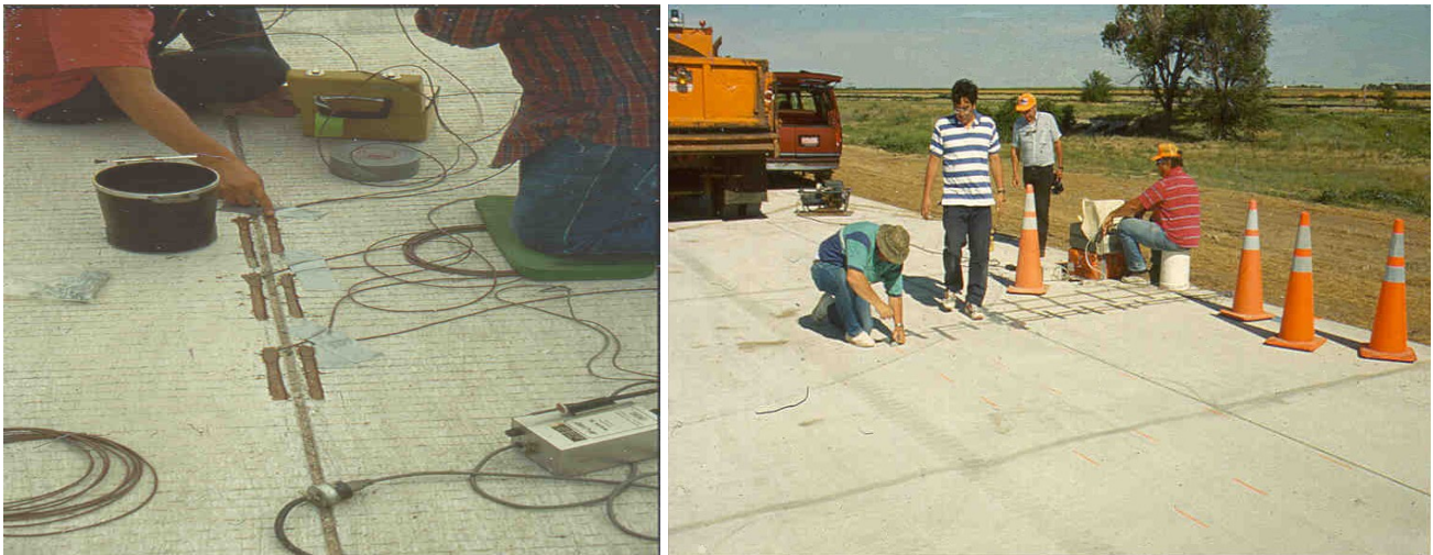
Figures 19 and 20: Surface Mounted Strain Gauges
