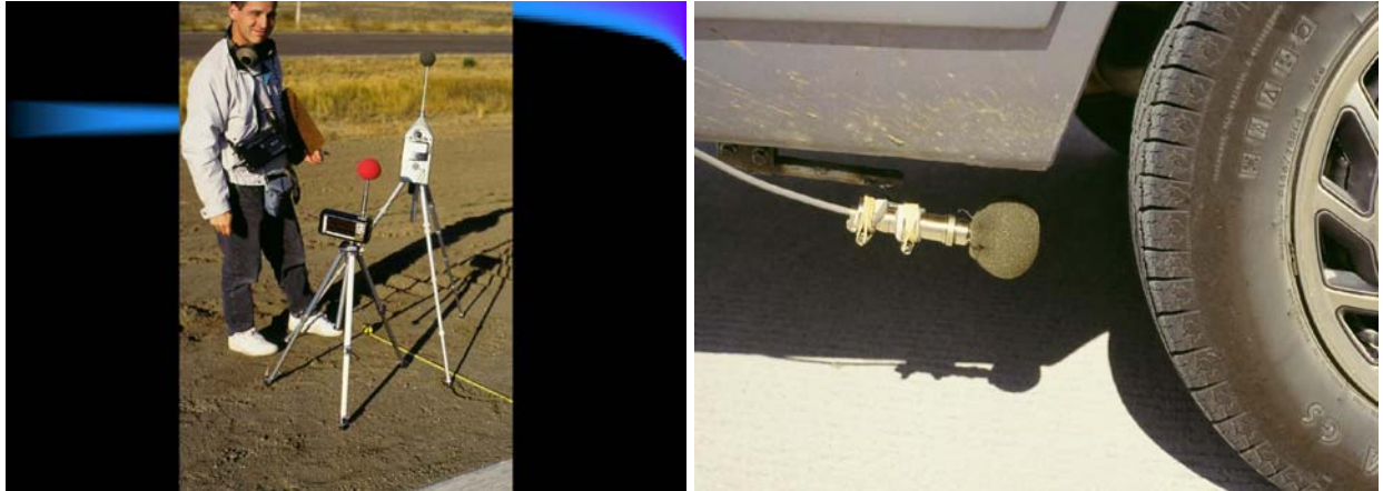
Figure 9: SPL Measurements at Roadside and Behind the Rear Tire
