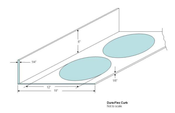
Figure 16. Drawing of the modified DuraFlex Curb used on US-50.
