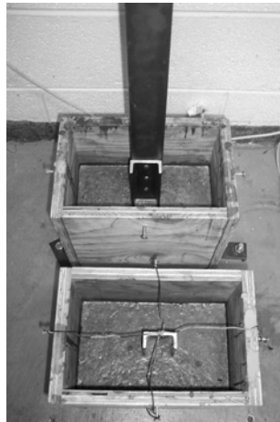
Figure 6: Steel channels in fresh SCC
