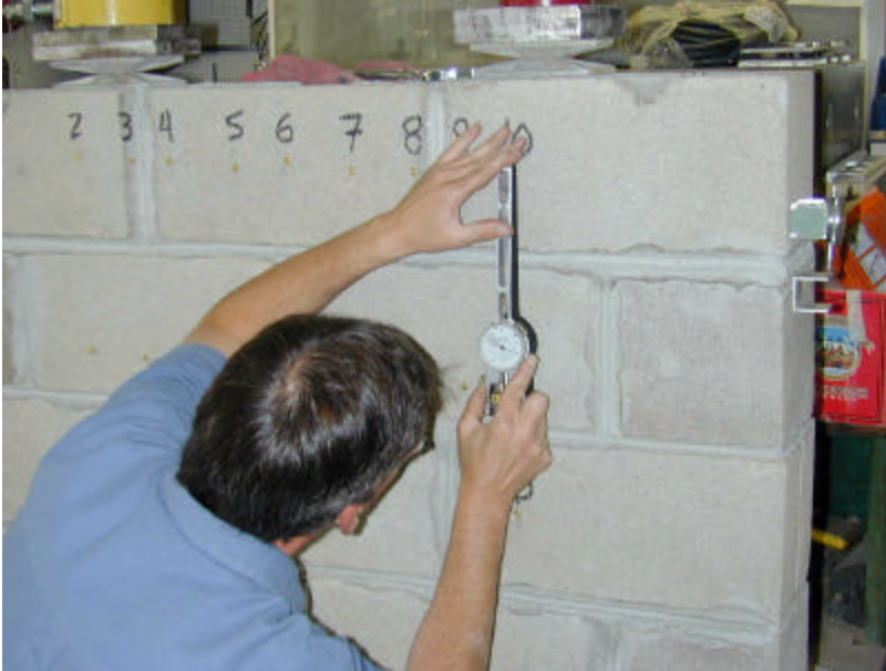
Figure 2. Laboratory tests of bond beam anchorage. The top course is a fully grouted, horizontally reinforced bond beam constructed with 8-inch concrete block. Strains were measured with a dial gage at 10 points between the two tendons (top of photograph).
