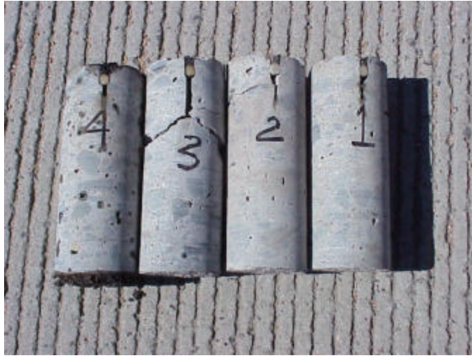
Figure 9. Cores from the non-working shoulder joint on I-70 at Deer Trail.
