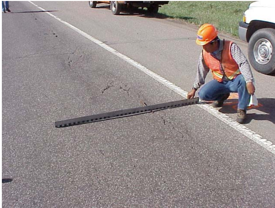
Figure B.3. Rutting Measurements on Existing Asphalt Pavement
