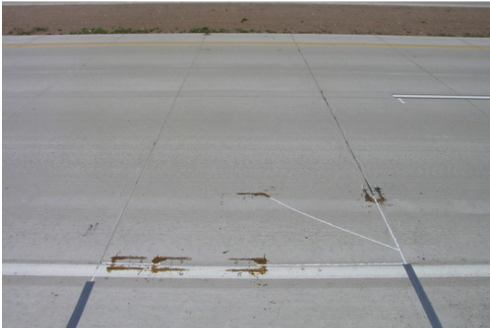
Figure D.7. Typical Test Slab with Surface Gages Installed
