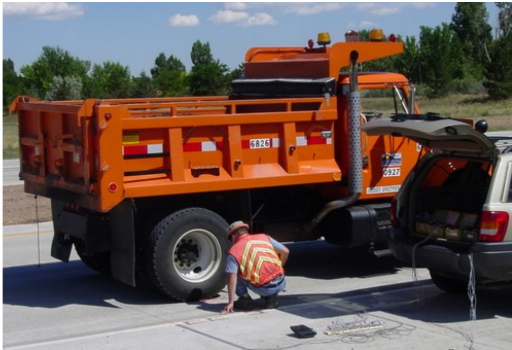
Figure 4.3. Truck Wheel Placement During Load Testing
