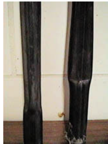
Figure 23: Crushed CFRP Grips
