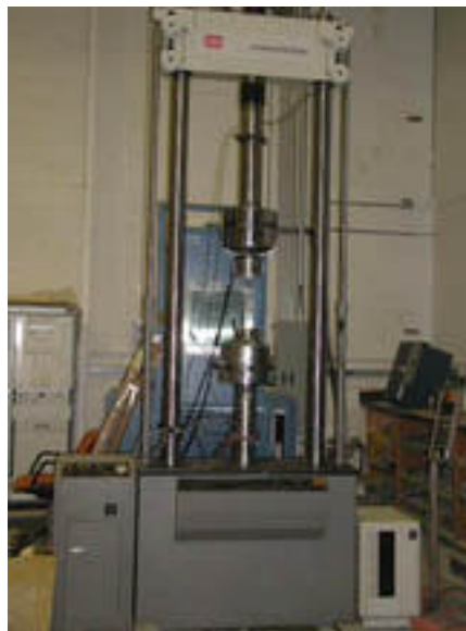
Figure 25: MTS Testing Apparatus
