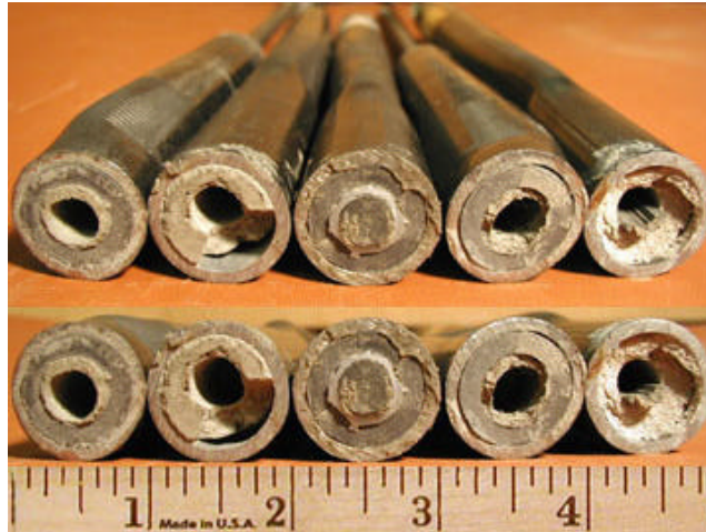
Figure 24: Unconditioned CFRP Grip Failure
