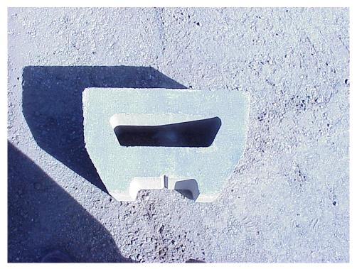
Figure B-9. Bottom view of Mesa block showing smooth flat surface with no grooves or
