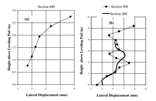
Figure 11. Lateral displacements monitored on phase I structure: (a) during stage I construction, and (b) due to placement of the bridge superstructure.
