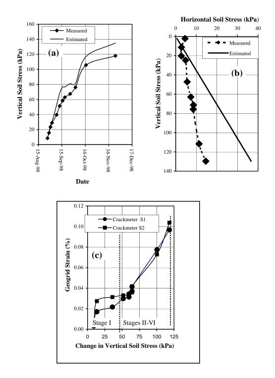
Figure 10. Measured and estimated data on section 400 of the phase I structure: (a) Vertical Stresses, (b) Horizontal Stresses, and (c) Geogrid Strains.
