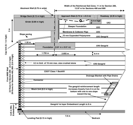
Figure 3. Typical monitored cross-section (sections 200, 400, and 800 in Figure 2) through the front and abutment MSE walls.
