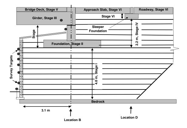
Figure 8. Instrumented section 200 indicating construction stages.
