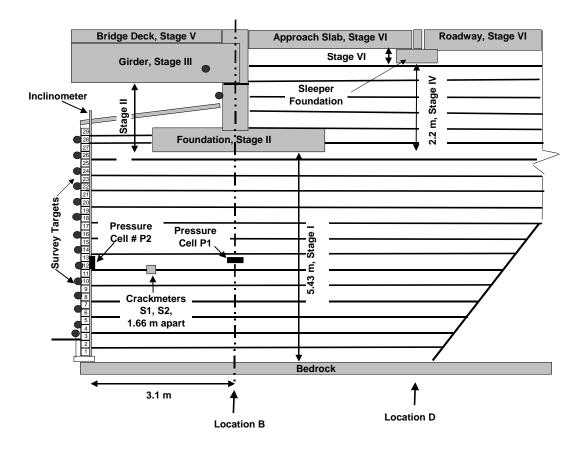
Figure 9. Instrumented section 400 indicating construction stages.
