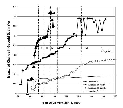
Figure 14. Measured geogrid strains during all construction stages (measured on the 6<sup>th</sup> geogrid layer of section 800).
