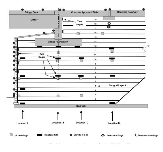
Figure 12. Instrumentation layout at section 800 (phase II structure).
