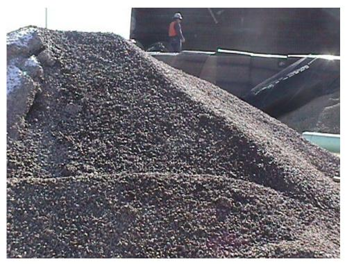
Figure B-6. The 19 mm maximum size crushed stone aggregate used to fill in and for .3 m behind the blocks to facilitate compaction and drainage behind the blocks, prevent washout of the fines in the fill material, and facilitate compaction behind the facing.
