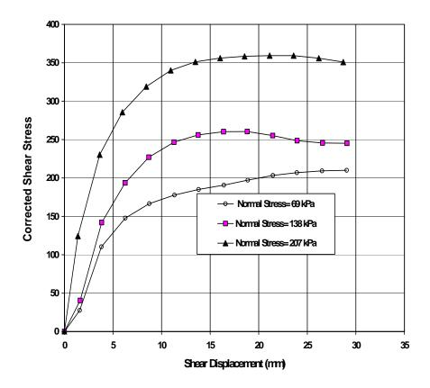
Figure 5. Results of large-size direct shear tests.
