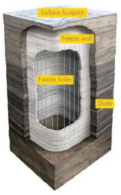
Graphic representations of Shell's In situ Conversion Process and freeze wall plans. Electric heaters gradually heat the shale underground until the oil is freed from the rocks and can be pumped to the surface. Around the extraction zone, the underground freeze wall is designed to protect groundwater against contamination. Credit: Shell Oil USA (used by permission)
