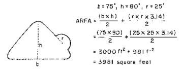
Figure 4: Area calculation for an irregular-shaped pond.
