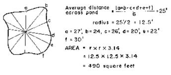
Figure 6: Area calculation for an irregular-shaped pond.
