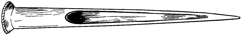
FIG. 1.—Seed trier which may be used in taking samples of the smaller seeds from sacks without opening the sacks.
