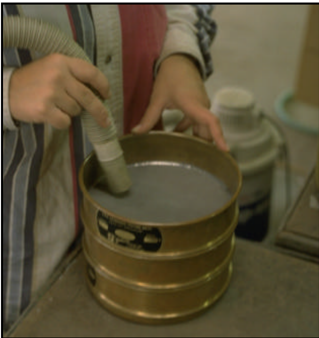
Figure 11: Three layers of soil sampling sieves and a blower are used to remove the seed from the cotton.
