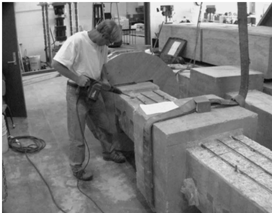
Figure 1-37 The surface of the FR specimen was roughened and prepared for shotcrete. The specimen was turned upside-down by rolling on large plywood wheels, like the one supporting the far end of the specimen, to avoid disturbing the shotcrete before it had fully cured.
