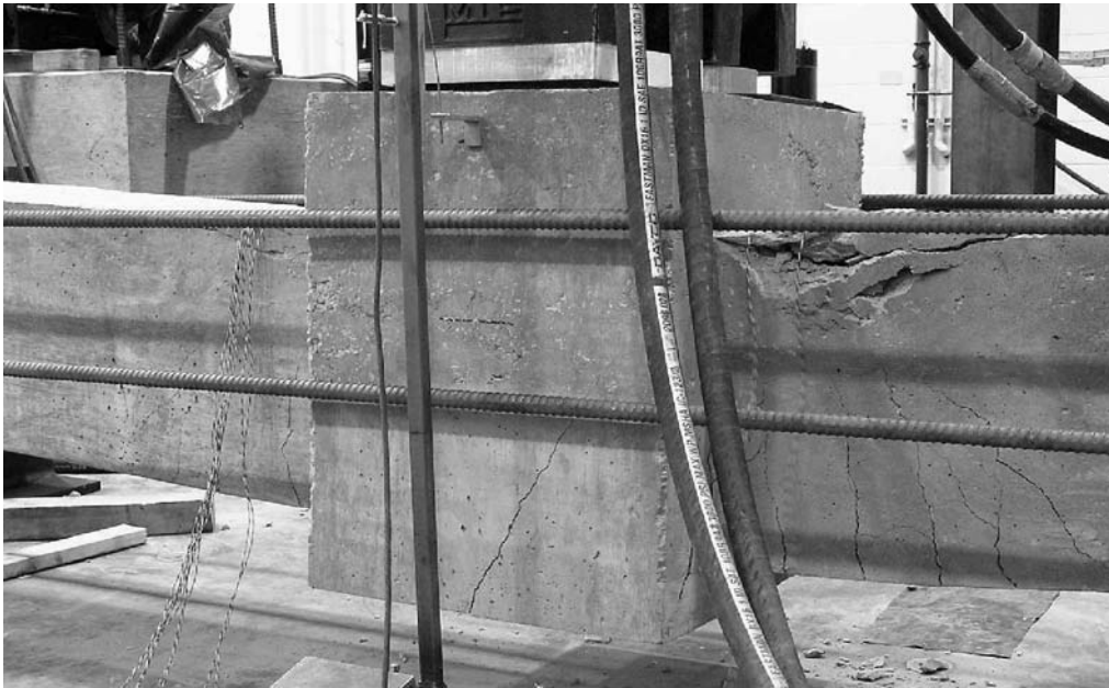
Figure 1-58 Cracking and spalling around central block (FC specimen)
