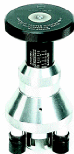
Figure 2-19 The pull-off test apparatus
