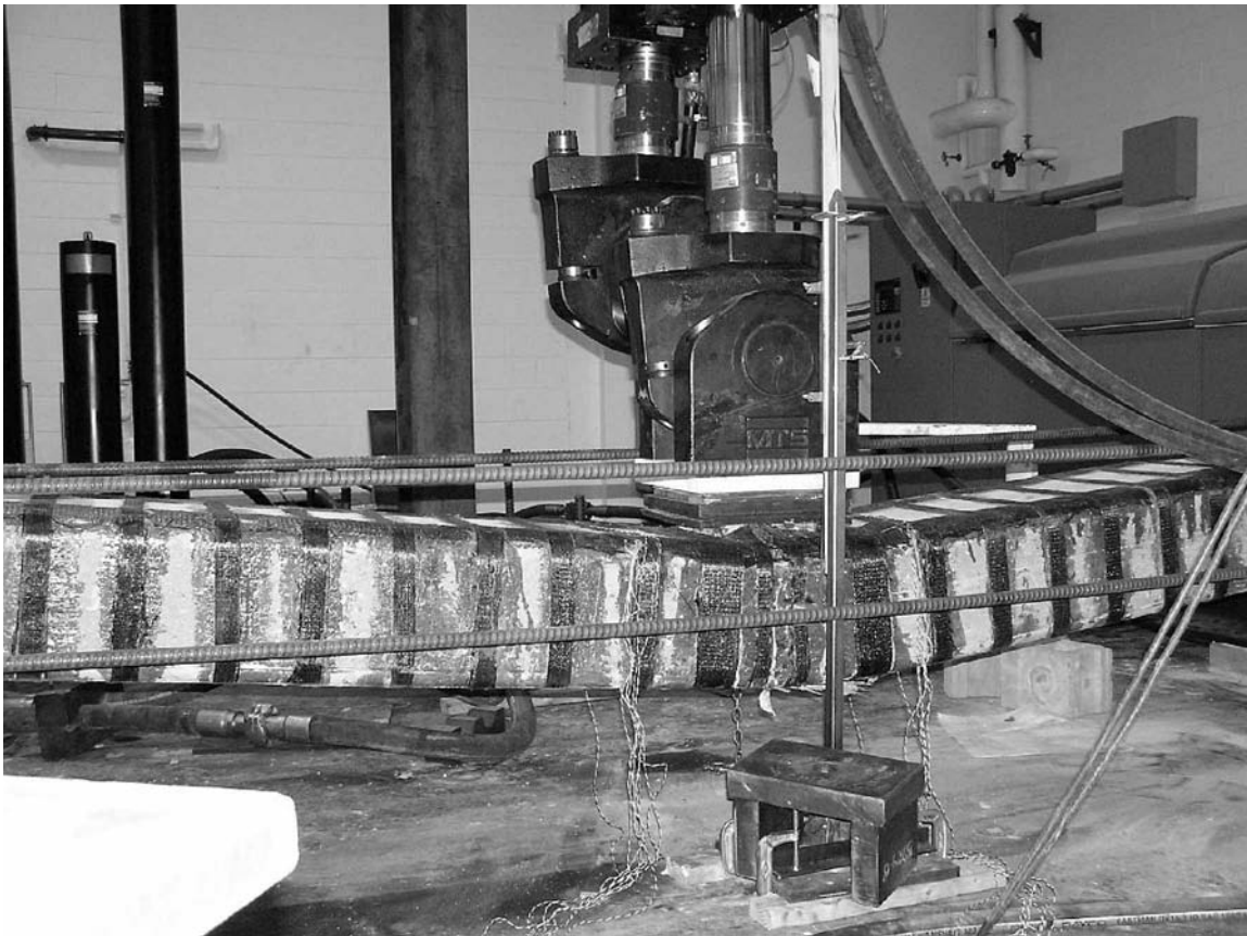
Figure 1-44 A single piston was used to apply the center load to the AR specimen. This picture was taken near the end of the test.
