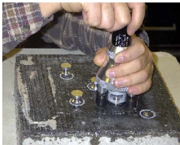
Figure 2-20 View of pull-off testing in progress
