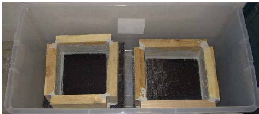
Figure 2-17 The ponded specimens in the bath
