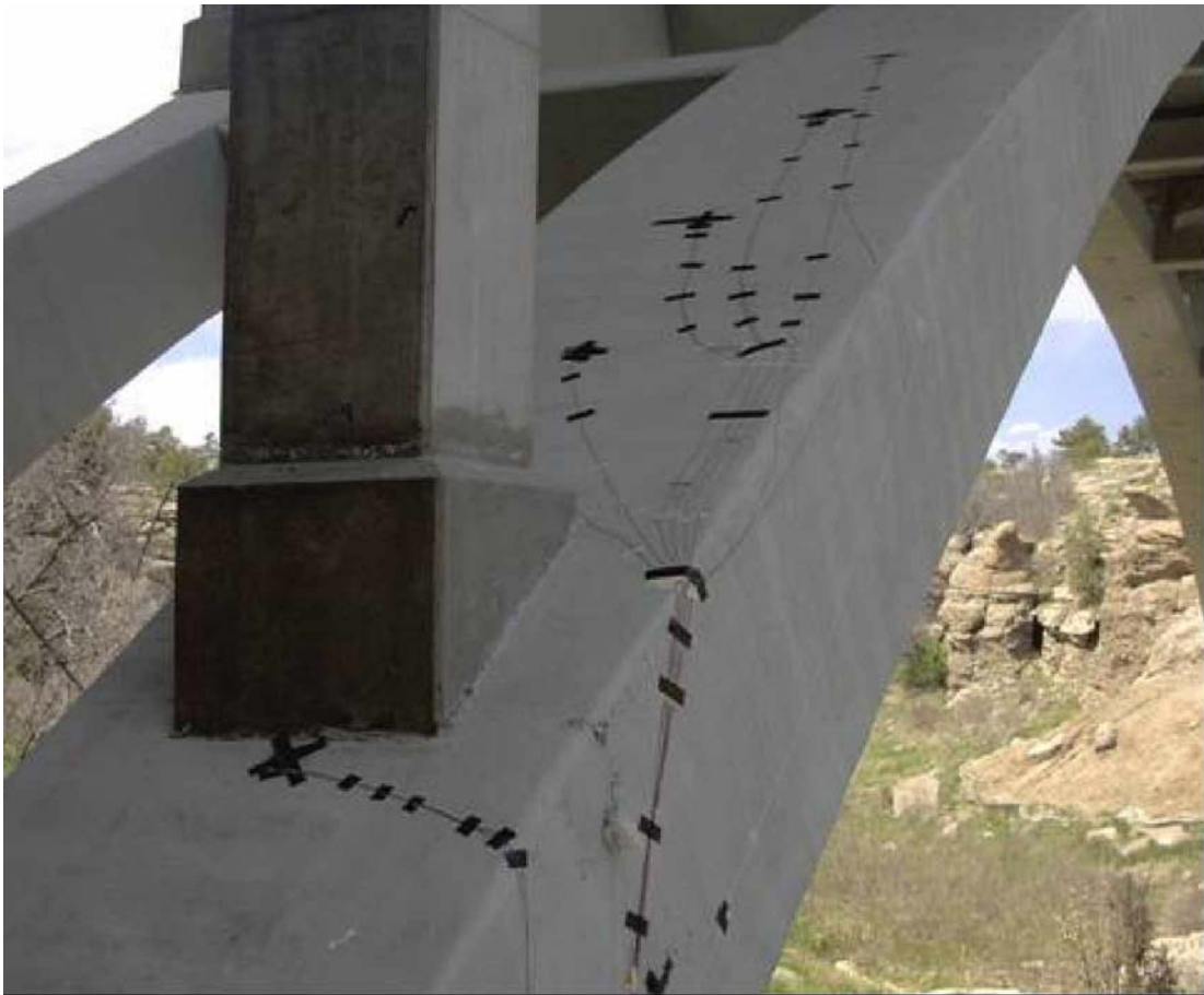
Figure 3-7 Wiring of strain gages - Extrados (Back)
