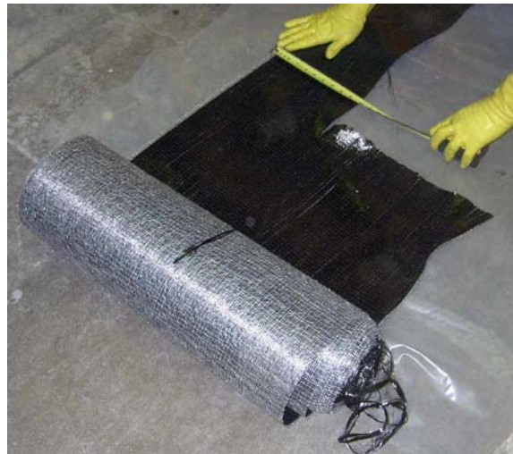
Figure 2-13 Tyfo SCH-41 roll sheet
