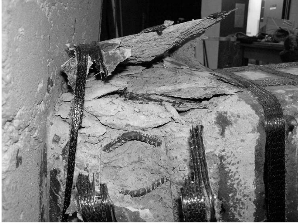
Figure 1-66 Compression region of the FR specimen critical section
