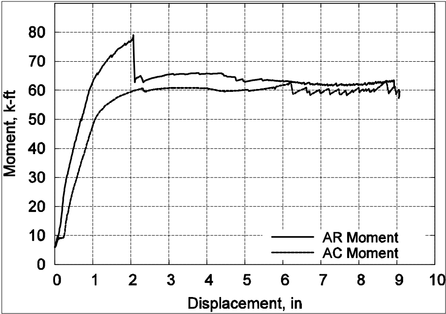
Figure 1-76 M vs. mid-span deflection for arch specimens
