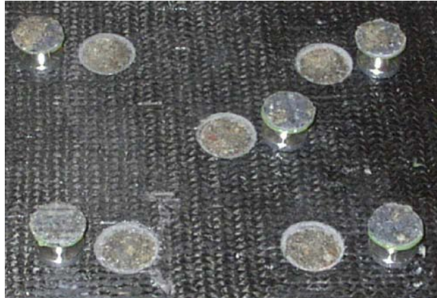
Figure 2-22 CFRP surface after a pull-off test
