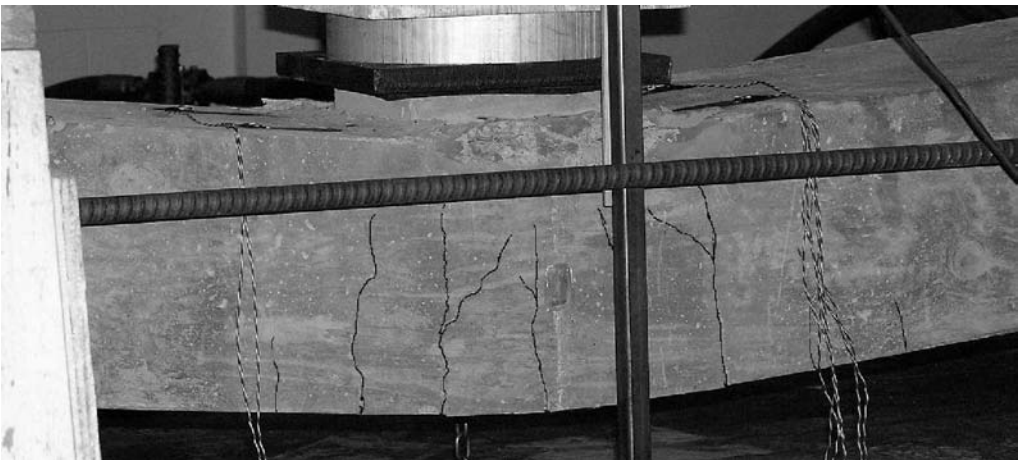
Figure 1-48 Crack pattern at end of test (AC specimen)
