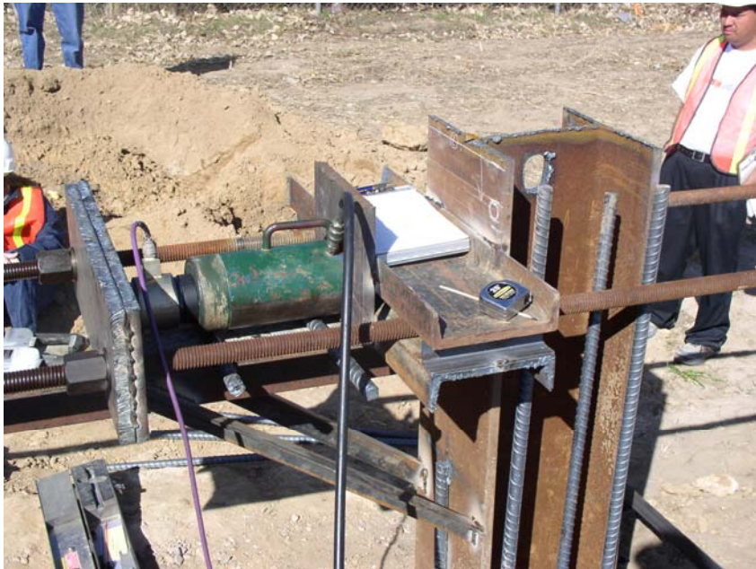
Figure 5.48 Picture showing the jacking devices
