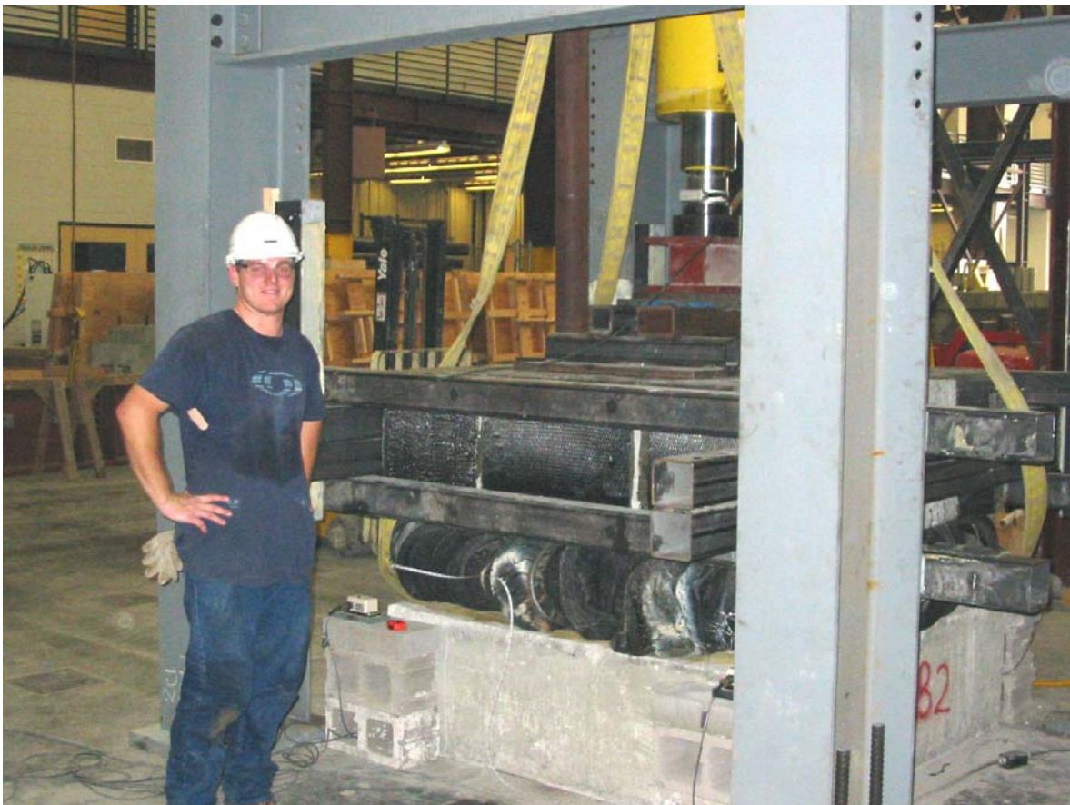
Figure 14: Tire Bale # 8 loaded to 592 kips
