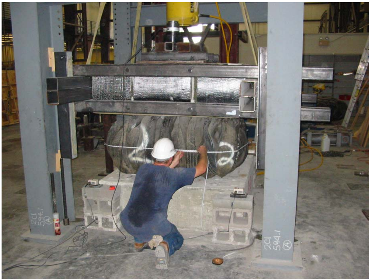
Figure 6: Circumferential measurements. Outriggers mitigated rotation problem.
