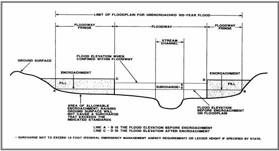
The floodway is defined by Federal Emergency Management Agency (FEMA) as the channel plus any adjacent floodplain areas, that must be kept free of encroachment so that the 100-year discharge can be conveyed with no more than one foot rise in the water surface above the base flood elevations (BFE). Encroachment into the
