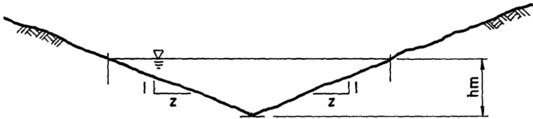
Figure II-8. Typical Urban Drainage Channel Geometry.
