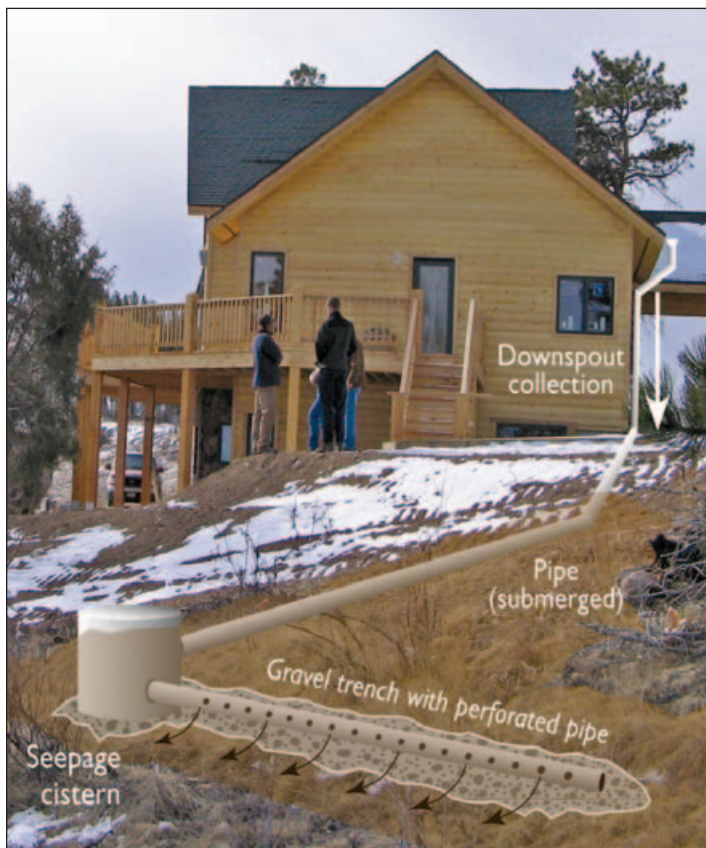
Subsurface infiltration techniques reduce runoff, erosion, and evaporative losses while maintaining predevelopment hydrology.
