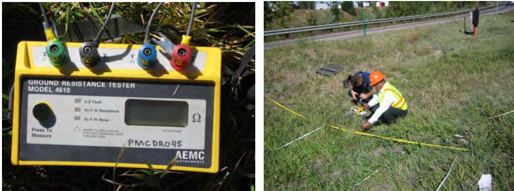
Figure 1. Soil resistivity testing by ASTM G57-95a
