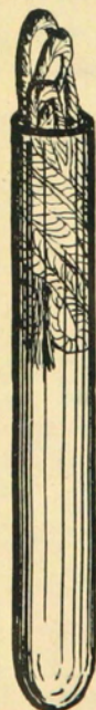
Figure 5.—Vial and cord for holding the liquid alcoholate used in making the test for carbon disulfide gas diffusion.
