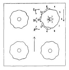
PLATE 4.—Suggesting a system of work in the orchard to develop thoroughness in spraying. The long arrows indicate the lines of movement of the machine. The man on the tower sprays from the positions of A, B and C, and repeats from similar positions when the machine is on the other side of the row. The figures indicate the spraying positions of the man on the ground. See the text for a more complete description.
