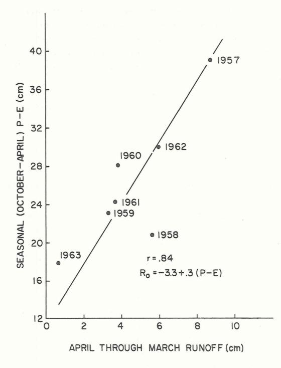
Figure 28. Seasonal (October through April) P-E computed from the atmospheric winter balance plotted against the April through March runoff at Lee's Ferry. The solid line is the linear regression fitted to the data.
