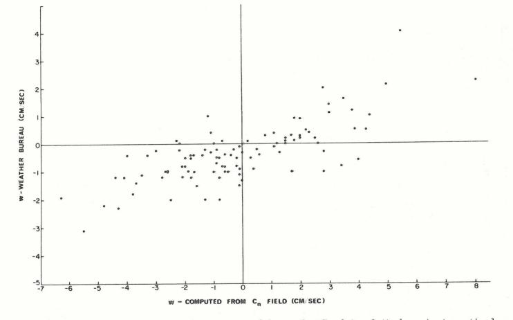
Figure 8. Vertical motion at 475 mb computed from the  $C_n$  data plotted against vertical motion at 500 mb putlished by the U.S. Weather Bureau.
