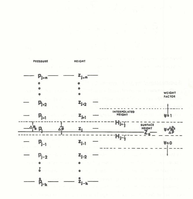
Figure 7. Scheme for obtaining weighting factors,  $\psi_{ij}$  .
