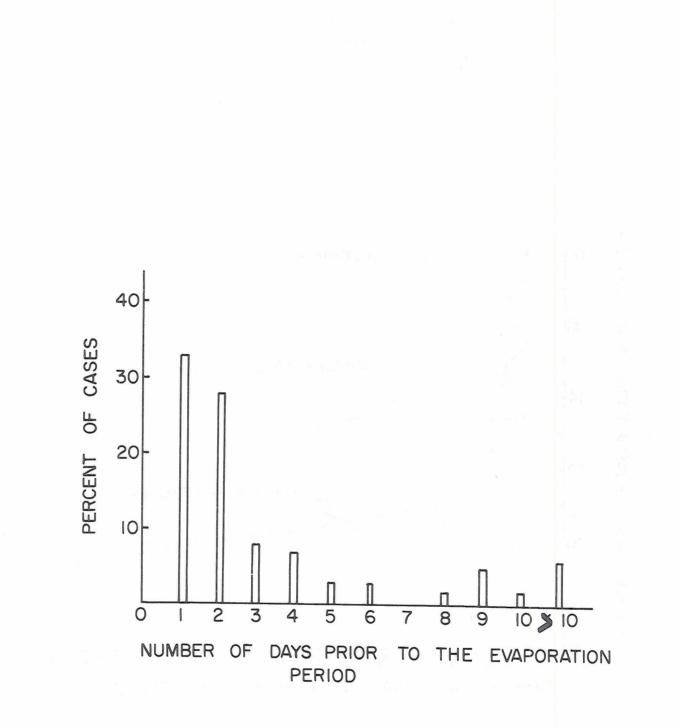
Figure 24. Days prior to evaporation period needed to accumulate the quantity of water evaporated during the evaporation period.
