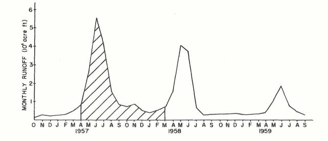
Figure 27. Solid line is the monthly course of runoff measured at Lee's Ferry, Arizona, for the water years 1957-1959. The hatched area is the amount of runoff assumed to be due to the October, 1956, through April, 1957, deposition.
