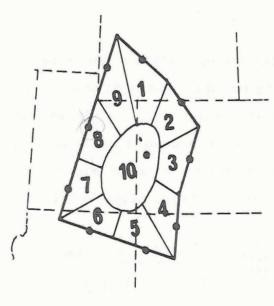
Figure 6. A rea increments used to obtain the area weighted averages.
