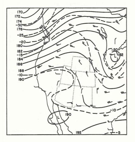
Figure 11. The 500 mb map for 26 October, 1960, 0000Z. Contours (solid lines) are in 100's of feet msl. Isotherms (dashed lines) are in degrees centigrade.
