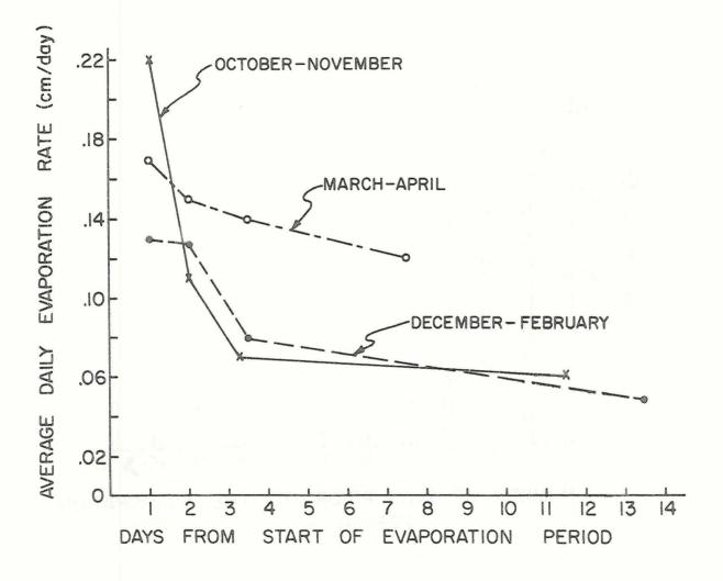
Figure 25. Decay of evaporation rate with time from start of the evaporation period.
