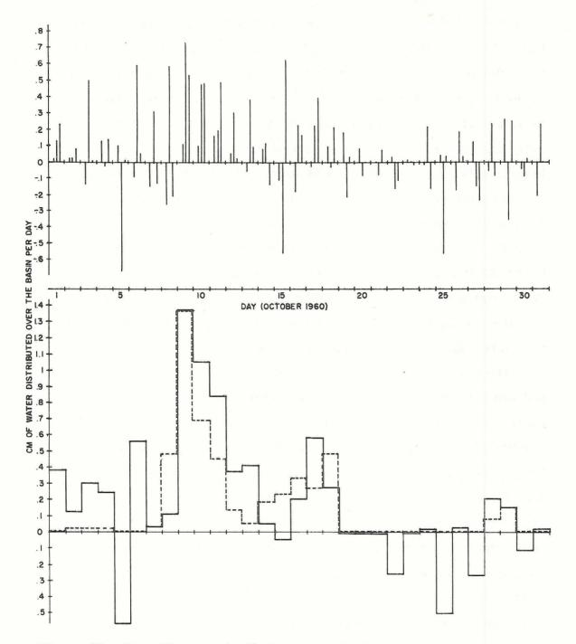
Figure 15. Top: The vertically integrated values of the three terms in the atmospheric water balance. For each day the three bars represent the local change (left), mean divergence of flux (middle) and the eddy divergence of flux (right) terms, respectively, a positive value indicates a positive contribution to the residual (P-E).
