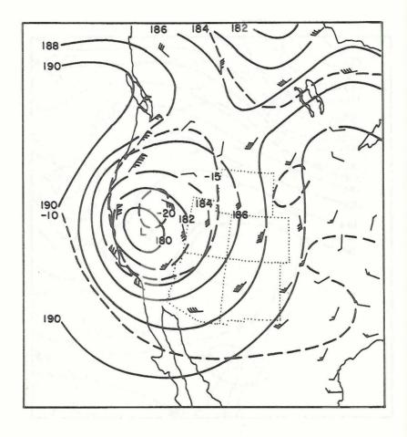
Figure 10. The 500 mb map for 10 October, 1960, 0000Z. Contours (solid lines) are in 100's of feet msl. Isotherms (dashed lines) are in degrees centigrade.
