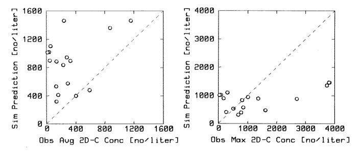
Figure 13. Observed average 2D-C ice crystal concentrations in the seeding curtains of 17 cumulus congestus clouds versus the model predicted values applying the laboratory effectiveness spectrum using the Holroyd et. al. (1978) sublimation rate formula.
