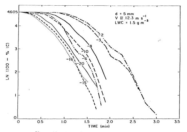
Figure 15. Composite kinetics plots for 5 mm dry ice pellets over a range of temperatures. The plots for -5, -9, and -12 <sup>O</sup>C have not been included in order to reduce confusion in the figure.
