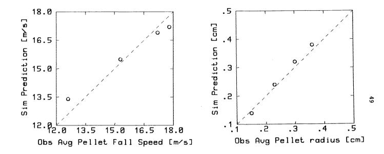
Figure 10. Observed dry ice pellet fall speeds from clear air drop experiments versus simulation prediction.
