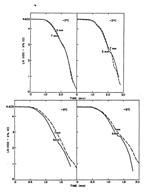
Figure 17. Composite kinetics plots for 5 and 7 mm dry ice pellets for several warm temperatures at a cloud liquid water content of  $1.5 \text{ gm}^{-3}$ .
