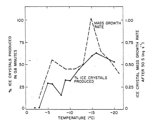
Figure 16. Percentage of the total number of ice crystals counted that were observed in 0.8 minutes for 5 mm dry ice pellets at a cloud liquid water content of 1.5 g m<sup>-3</sup> (solid line). The pellets velocity was 12.3 m s<sup>-1</sup>. The mass growth rate for ice crystals after Ryan <u>et</u>. <u>al</u>. (1976) is plotted as the dashed line.
