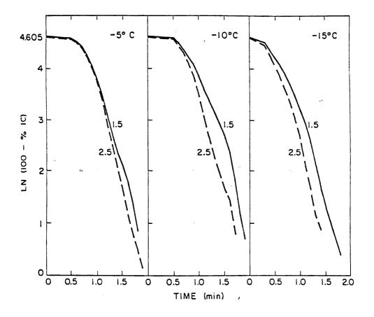
Figure 19. Composite kinetics plots for 5 mm dry ice pellets at 1.5 and 2.5 g m<sup>-3</sup> cloud liquid water contents. Pellet velocities are approximately 12.3 m s<sup>-1</sup>.
