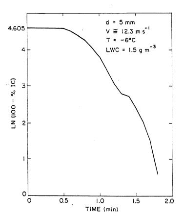
Figure 9. Composite kinetics plot formed from the plots in figure 8.
