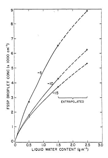
Figure 18. Extrapolation of cloud droplet concentrations for -5, -10, and -15  $^{\circ}$ C at a cloud liquid water content of 2.5 g m<sup>-3</sup>. The data points at 0.5 and 1.5 g m<sup>-3</sup> were taken from figure 3. The curves shown are hand-fitted.
