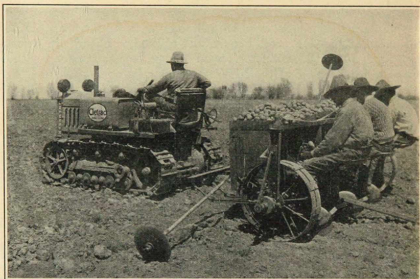
Fig. 37. Three-row cup-type planter and men to correct the feed.
