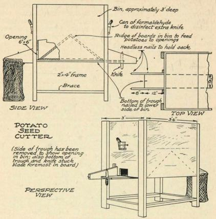
Figure 49. This cutting box makes potato cutting a lighter job.
