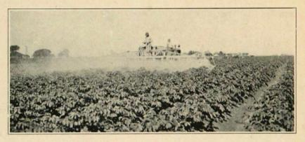
Figure 76. A six-row power take-off tractor sprayer in operation. Three hundred pounds' pressure is recommended.
