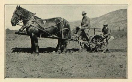
Figure 18. A potato planter equipped with a commercial fertilizer attachment. Commercial fertilizer gives best results when placed in bands a little below and to each side of the seed piece.
