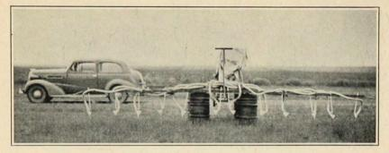
Figure 77. A six-row power take-off tractor duster. This machine is adapted to the dry lands, as it eliminates the cost of hauling water.
