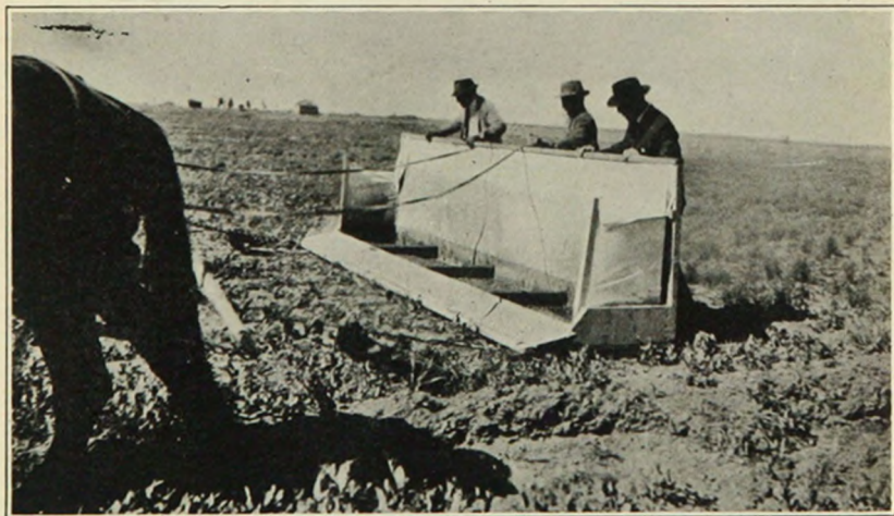
A 'hopper dozer' in action. One of the many machines that was used in the grasshopper campaign, 1916, San Luis Valley. (Colorado Experiment Station Bulletin No. 233.) Jones.
