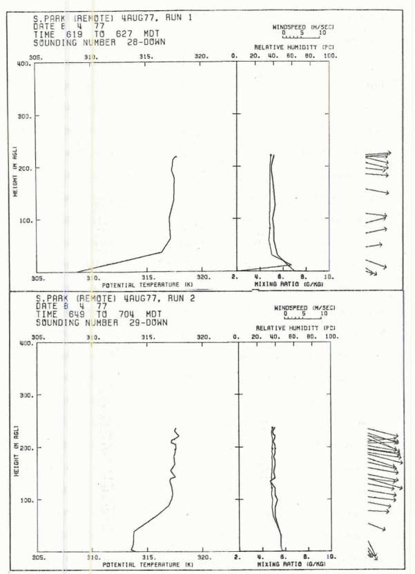
Figure 47. Boundary Layer Profiler (BLP) tethered balloon soundings. Potential temperature, water vapor mixing ratio, and winds plotted against height in meters AGL. Soundings begun at a) 0619 MDT, and b) 0649 MDT, 04 August 1977, both at Site #2. Y
