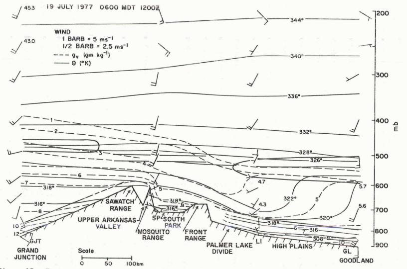
Figure 17. East-west cross-section including soundings from Grand Junction (GJT), South Park (SP), and Limon (LI), Colorado and Goodland (GL), Kansas. Solid contours are potential temperature (°K) and dashed contours are water vapor mixing ratio (gm kg<sup>-1</sup>). Terrain elevations and stable layer boundaries are marked with bold lines. Valid for 0600 MDT, 19 July 1977.
