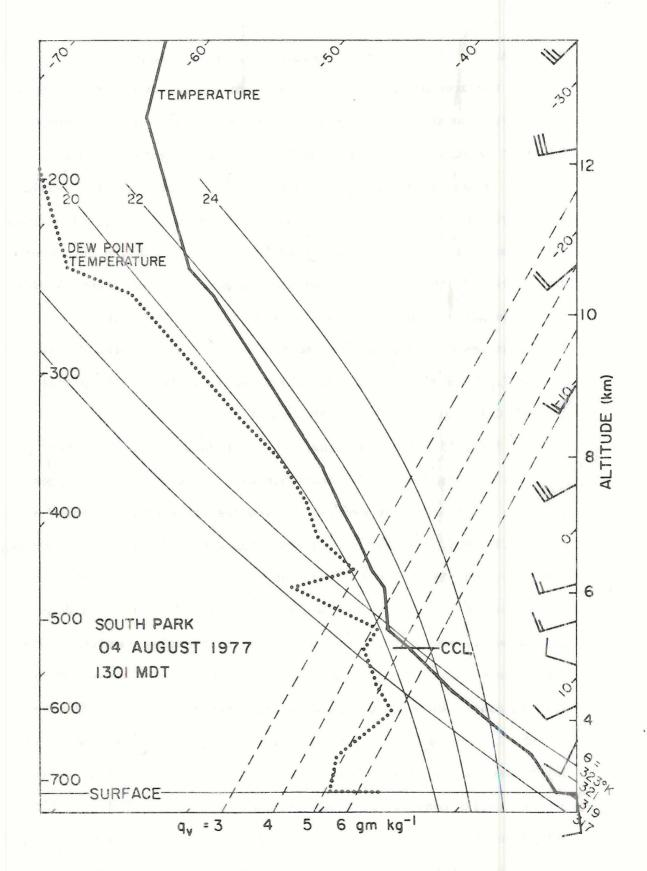
Figure 55. South Park sounding of 1301 MDT, 04 August 1977, plotted on skew-T log-P diagram. Cloud Condensation Level (CCL) marked.
