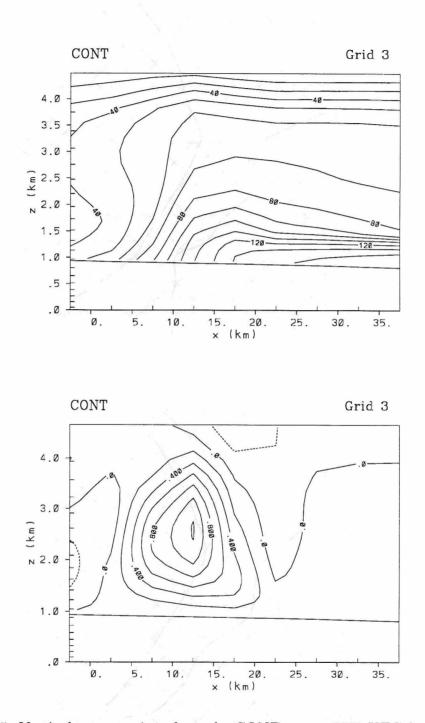
Figure 2.15: Vertical cross sections from the CONT run at 0000 UTC for a transect shifted 20 km from the transect depicted in Figure 2.13. The top panel is an analysis of water vapor mixing ratio (dg kg<sup>-1</sup>), and the bottom panel is for vertical motion (m s<sup>-1</sup>).
