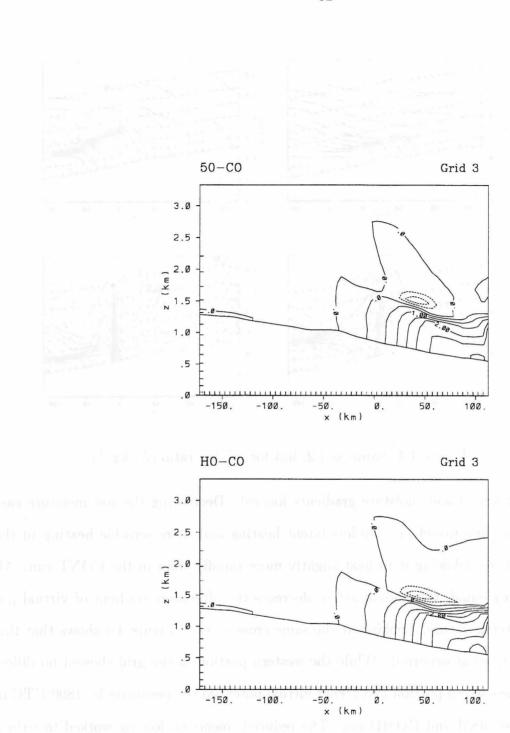
Figure 4.4: 50SM minus CONT (top) and HOMD minus CONT (bottom) virtual potential temperature difference (K) at 1800 UTC for same cross section as 4.1. Contour interval of 0.5 K.
