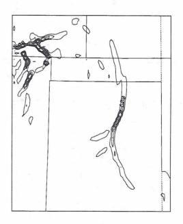
Figure 4.13: Same as 4.9, but for upward vertical velocities greater than 0.1 m s<sup>-1</sup> at approximately 1500 m AGL. Contour interval of  $0.5 \text{ m s}^{-1}$ .
