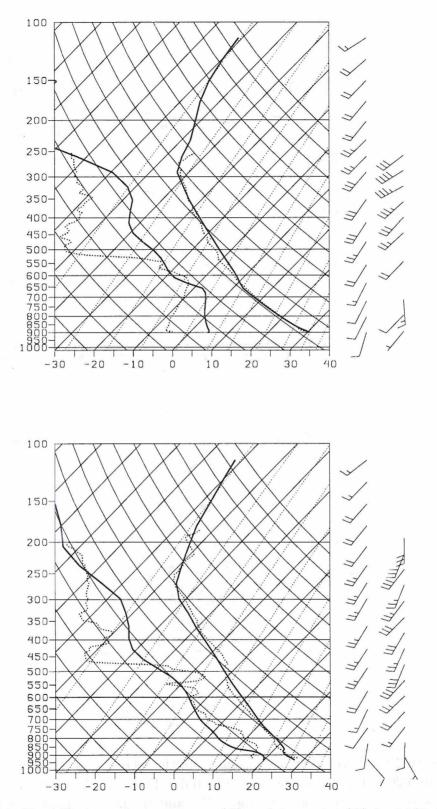
Figure 2.14: Skew-T plots of temperature (C) and dewpoint (C) for MC1 (top) and MC2 (bottom). Solid lines are from CONT run closest grid point. Dotted lines are the observed profiles. Left and right wind profiles are from the CONT run and observations, respectively. Winds in m  $s^{-1}$ .
