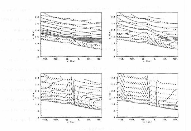
Figure 4.2: West to east vertical cross section of virtual potential temperature (K) on grid 3 at 1500, 1800, 2100, and 0000 UTC for the CONT simulation. Cross section taken at same latitude as P-3 transect, averaged over 6 points in the north-south direction. Longest vectors are approximately 20 m s<sup>-1</sup>.
