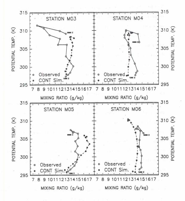
Figure 2.16: Conserved variable time series diagrams for four observation sites east of the dryline comparing observations to model grid point data.
