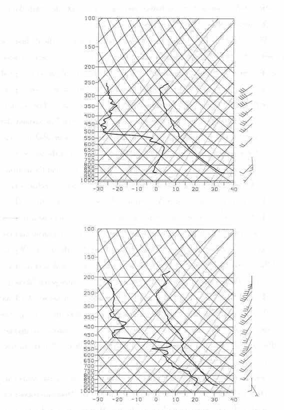
Figure 2.4: M-CLASS soundings from west of dryline (top) and east of dryline (bottom) around 2300 UTC.
