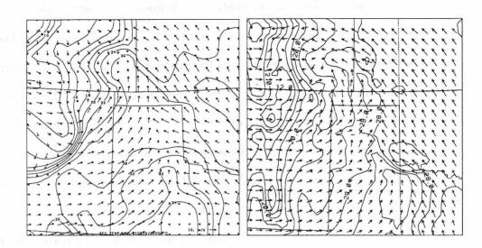
Figure 2.11: Objective analysis of temperature (contour interval of 2°C) and wind vectors as observed (left) and for the CONT simulation (right) at 0000 UTC, 16 May 1991. Vectors are of similar scale on the two plots. A reference vector is included in the lower right corner of the left panel.
