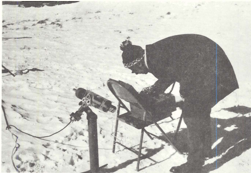
Fig. 4. Recording pyrheliometric observations
