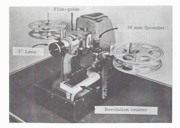
Figure 15. The snow crystal replica film-strip projector
