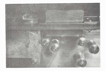
Figure 6. Snow crystal sampling slit and 35 mm film transport mechanism passed the coating wheel
