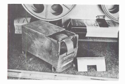
Figure 5. Formvar reservoir and "roll-on" coating wheel
