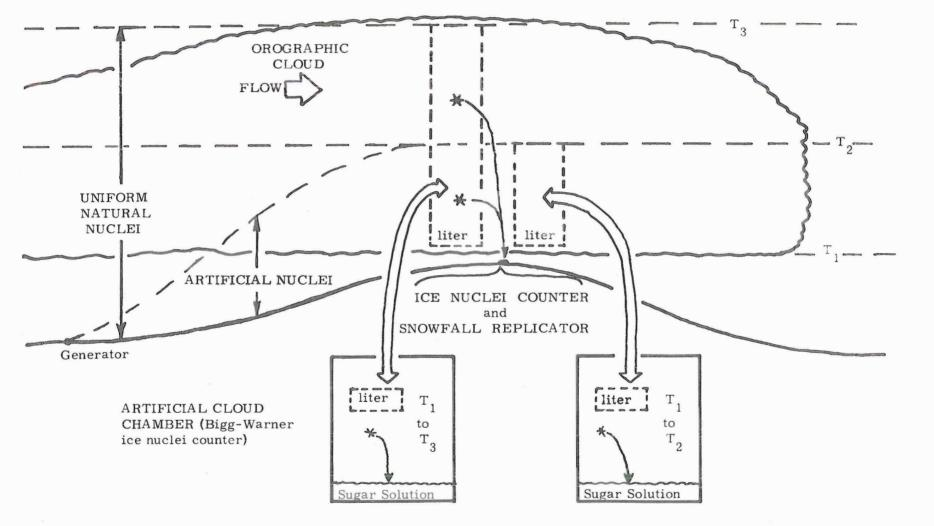
Figure 3. Schematic diagram of a simplified orographic cloud
