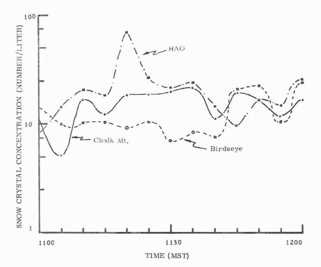
Figure 10. Comparison of total snow crystal concentrations observed by three simultaneously-operating replicators, Climax, Colorado, 27 December 1966
