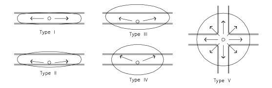
Figure 16. Horizontal distribution diagrams of Type I through V reflector distributions.<sup>6</sup>
