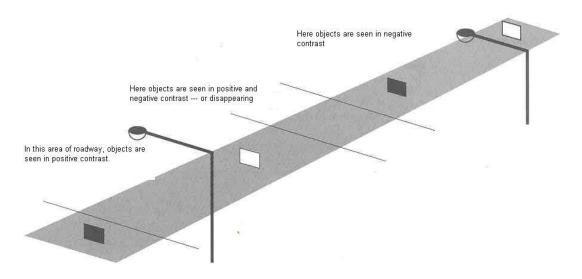
Figure 9. Objects along a roadway with positive, negative, and no contrast.<sup>3</sup>
