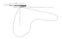
Figure 15. Vertical distribution diagram of a full cutoff luminaire.
