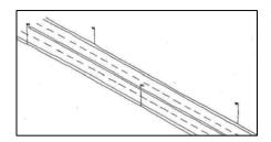
**Figure 14. Staggered configuration**
