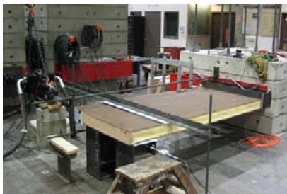
BioSIP test panel set up for racking shear load testing at CU’s Fast Hybrid Testing Lab.
