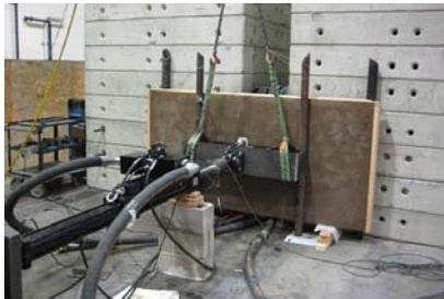
BioSIP undergoing the transverse bending load test.
