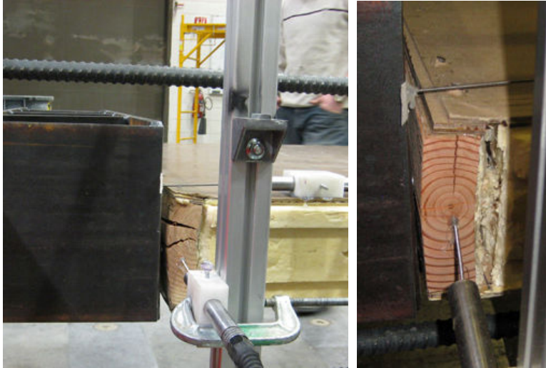
Photo 3.4: BioSIP Racking #2 test prototype shown in testing-to-failure of sill plate assembly (left). BioSIP Racking #1 prototype shown in testing-to-failure of sill plate (right).
