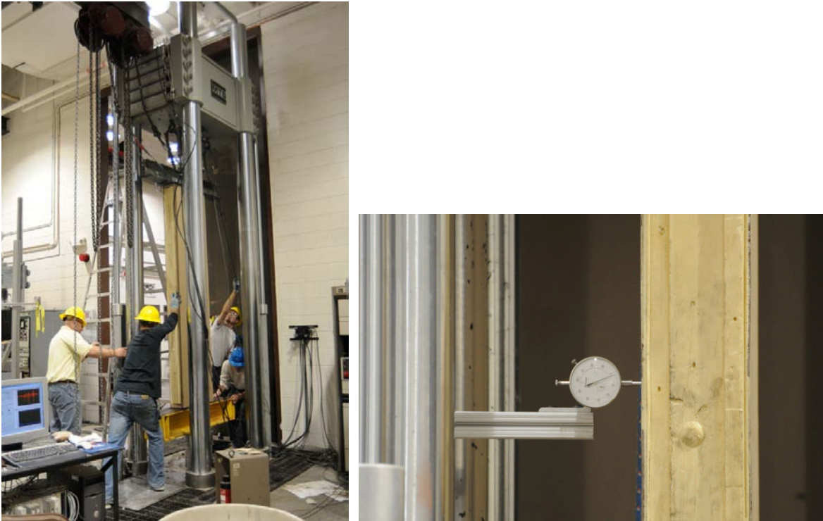
Photo 1.1 BioSIP axial test sample being loaded into MTS 1000-kip universal testing machine (left). Dial micrometer measuring BioSIP deflection at mid-height (right).
