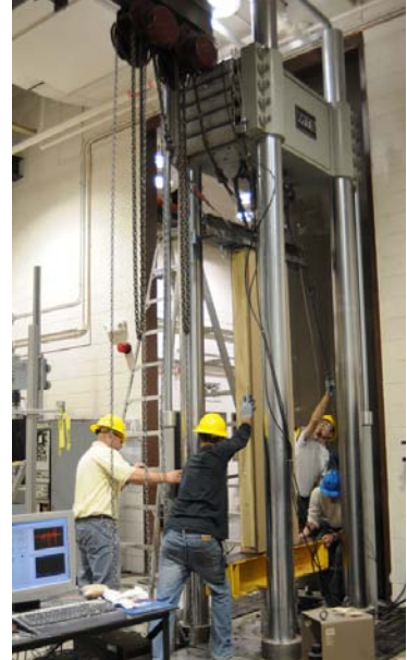
Loading a BioSIP test panel into the axial compression testing equipment
