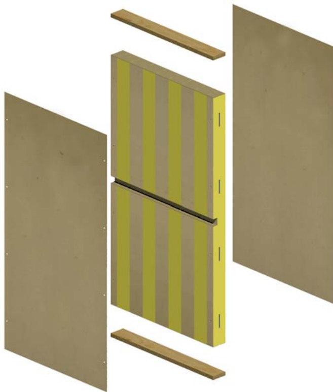
BioSIPs with structural 3D core encapsulated in high r-value insulation (R-7 per inch)
