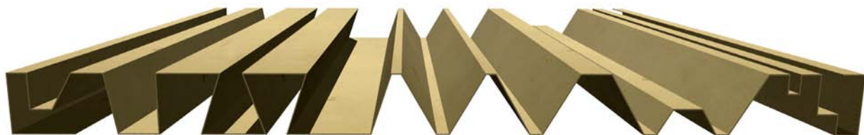
Computer model of a 3D EMF corrugated substrate.
