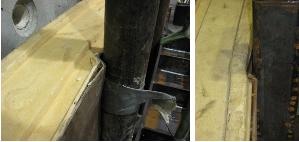
Photo 2.4: Close-up of BioSIP prototype at testing-to-failure position for Bending #3 (left) and Bending #2 (right).
