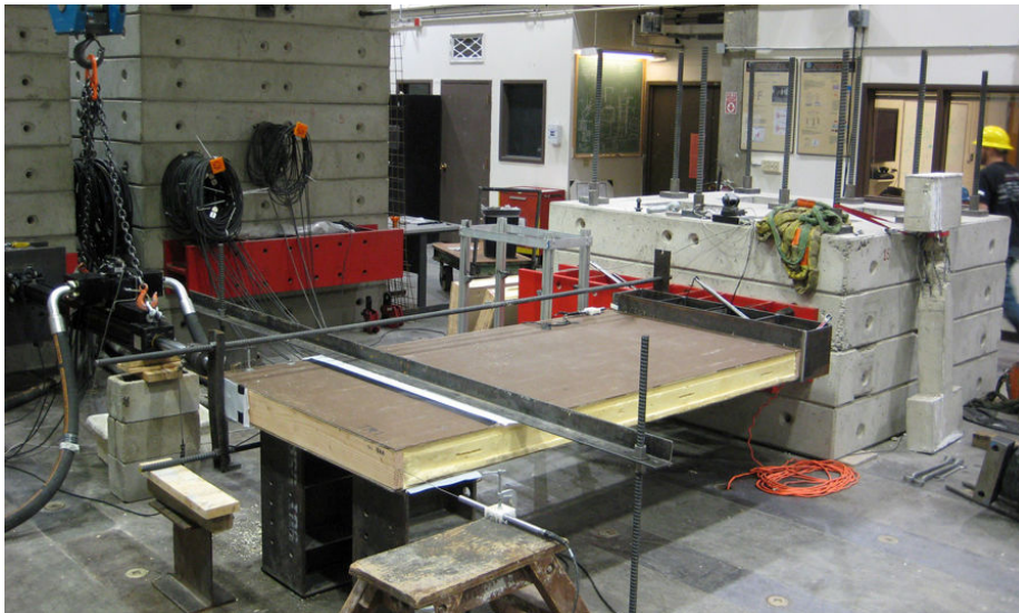
BioSIP prototype set up for racking shear load testing at CU's Fast Hybrid Testing Laboratory, January 2010
