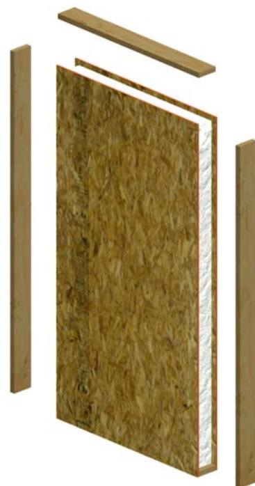
Standard sandwich panel SIP with two layers of OSB sandwiching a layer of expanded polystyrene insulation (R-3.5 per inch)
