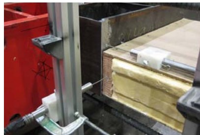
Strategically placed sensors were used to monitor results of the structural testing.
