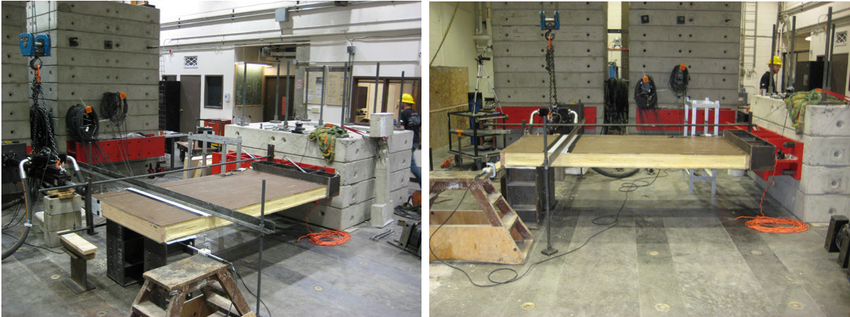
Photo 3.2: BioSIP prototypes shown in Racking #2 shear test configuration.
