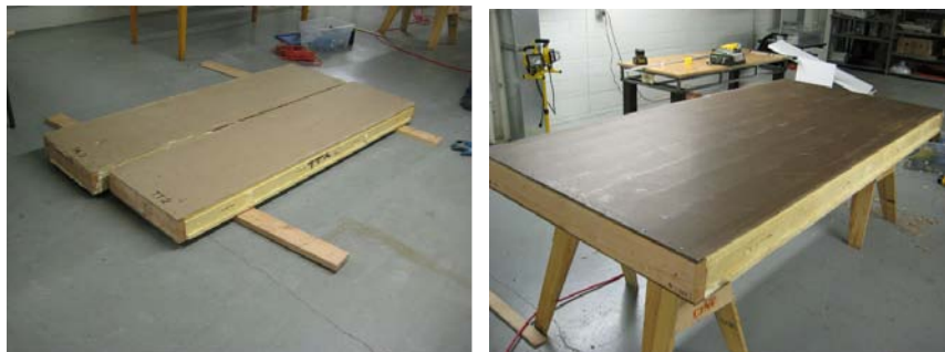
Photo 0.1: Example BioSIP physical testing prototypes as follows: 24"x96" prototype (left) and 48"x96" prototype.
