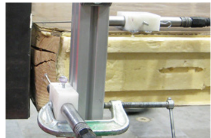
Detail view of the failure location along wood sill plate attached to the BioSIP test panel.
