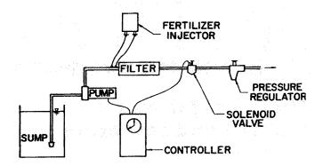
Figure 2: Typical trickle system "head."
