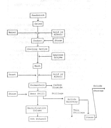
Figure 1. Alcohol production flow chart (190 proof ethanol).
