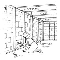
Cut blankets into sections long enough to extend from the top plate to 2 feet (.6 m) below the ground line. Staple them into place between the studs, with the vapor barrier towards the living space. Note: In mountainous regions there will be added benefit to installing the insulation the full height of the wall.
