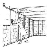
Install another small piece of insulation above the furring and against the sill to insulate the sill and band joist.
