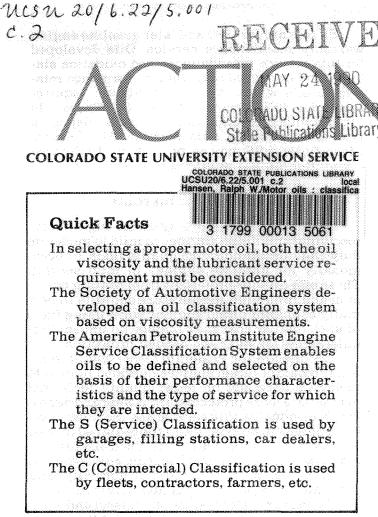
In selecting a proper motor oil, both the oil viscosity and the lubricant service requirement must be considered.
