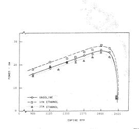
Figure 1: Gasoline engine full throttle power output using ethanol fuel blends.
