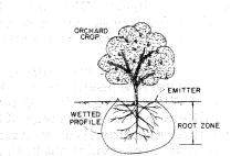
Figure 1: A wetted profile develops in the root zone below each "emitter" or "trickler."
