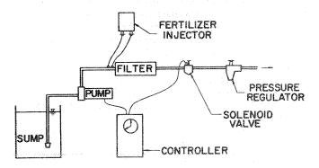
Figure 2: Typical trickle system "head."
