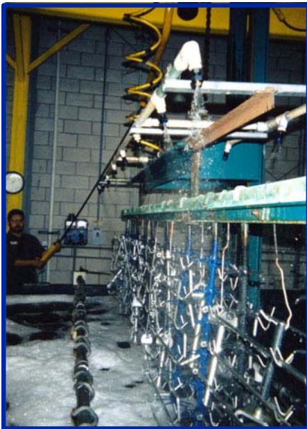
Hoist Mounted Spray System
