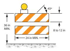
TYPE II BARRICADE Note: Warning lights optional Using Type III Barricades
