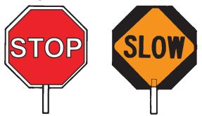
The STOP/SLOW paddle may be modified to improve conspicuity by incorporating either white or red flashing lights on the STOP face, and either white or yellow flashing lights on the SLOW face. The flashing lights shall be arranged in accordance with the most current MUTCD.
