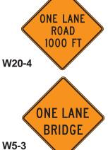
**ONE LANE ROAD SIGN (W20-4)** <u>This sign is frequently used to pinpoint areas</u> <u>where traffic traveling in both directions must use a single lane.</u> Traffic is moved through the area in one direction at a time. Pilot cars, convoy systems, double flaggers an AFAD device, or temporary traffic signals can be used to handle the situation. You will read more about pilot cars and convoy systems later.
