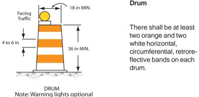
Because drums are bulky, and sometimes are heavy, they are used most often on projects which are of long duration. They also require much more room than cones. <u>Therefore,</u> generally speaking, drums are not used often on routine maintenance project or projects of short duration. This is because barrels are heavier than cones, and lack the portability of cones.
