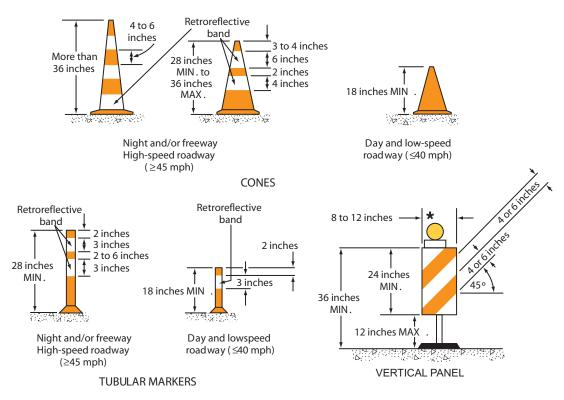
Devices used to channelize pedestrians shall be detectable to users of long canes and visible to persons having low vision.
