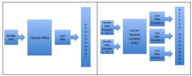
Figure 8: Current single provider model Vs. Carrier neutral location model
