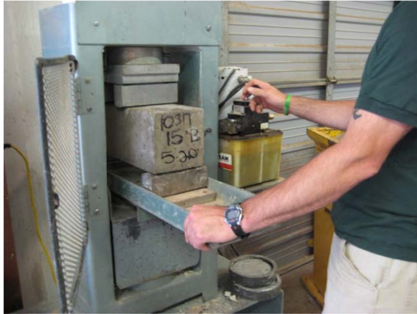
Figure 3.1. Flexural Strength Testing.
