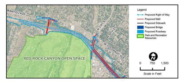
The grade separation of Ridge Road would improve safety for non-motorized travelers. The overpass structure would be approximately 27 feet high and 136 feet wide and would be visible from portions of the park. This would constitute a change in the visual environment, but would be consistent with the existing highway corridor. Noise levels could increase as a result of the wider roadway footprint and elevated structure.
